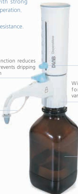
Fast, reliable and reproducible volume locking mechanism
