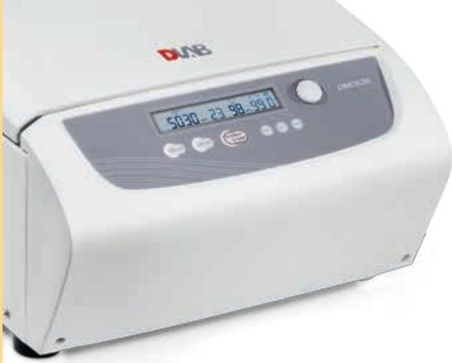
DLAB DM0636 Multi-Purpose Low-speed Centrifuge is ideal for the centrifugation of samples in clinical chemistry, cytology, research laboratories, industrial laboratories, etc. This centrifuge is suitable for tubes with caps, blood collection or urine tubes. Swing-out bucket rotors and adapters can be compatible with standard tubes up to 100mL at low speed.
