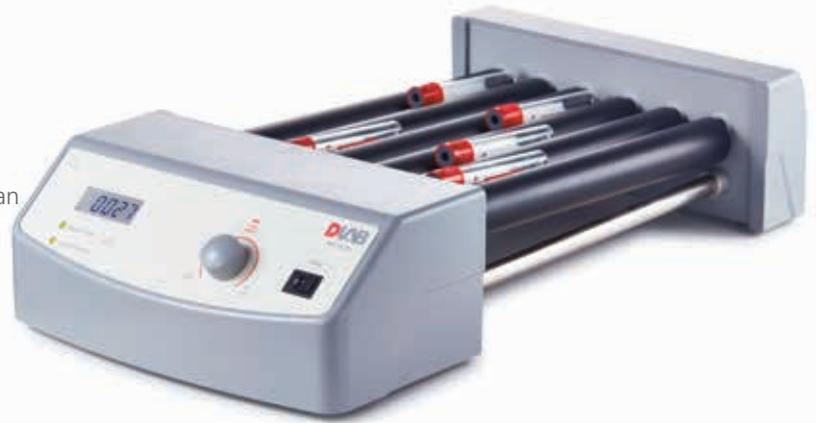
DLAB tube rollers provide a gentle and highly efficient rolling motions, ideal for mixing blood samples, viscous substances and liquid-solid suspensions. Used in a variety of applications, such as the prevention of blood coagulation, immune precipitation, etc.
